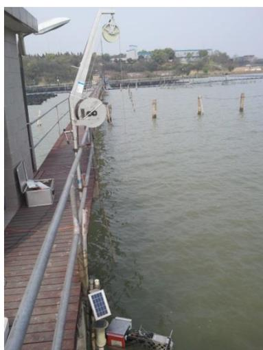
Figure V-4. MINIBAT long-term monitoring application in the shallow water Lake Taihu.
