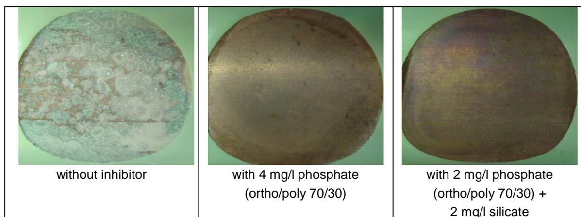
**Figure 10:** copper samples after cathodic polarisation
