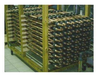
Figure 7 Test rig for the investigation of the copper surface and pit morphology After certain time intervals (often several weeks) one pipe of each string is taken from the test rig for investigation. The pipes are sliced horizontally and the surfaces are documented by photography.
