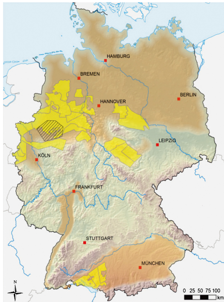
Figure 1 Mining authorizations in Germany (yellow, last revision: 31 December 2011) for exploration for unconventional hydrocarbon reservoirs (ochre: regions with the basic geological conditions for formation of shale gas) [1].
