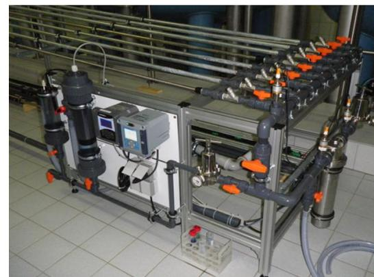
Test rig according to EN 15664-1
